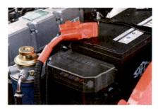
The forklift is now equipped with a next-generation integrated fuse box which makes maintenance and repair more convenient. The fuse box is laid out more intuitively and now offers better water-proof performance.
