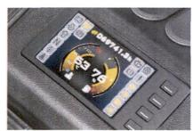
The newly-developed 4\* LCD instrument cluster has more comprehensive functions and offers more stable performance. The cluster displays the full truck state, fault codes, and other important information. This allows the operator to have a better understanding of the truck's state and makes maintenance convenient.
