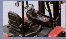
Extra foot space is provided to significantly reduce operator fatigue. The non-slip step makes getting in and out of the forklift easy and safe. A newly designed steering wheel new brake system, and easy-to-operate levers provide the operator with a comfortable operating experience.
